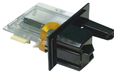
Payment Card Reader UIC payment device handles encryption, decryption
