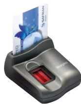
MorphoSmart 1350 USB Fingerprint Devices Feature Extractor Is MINEX/FIPS 201 Compliant
